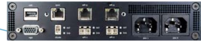
Identical interfaces on the sending side (Pitcher) and receiving side (Catcher) of the data diode
